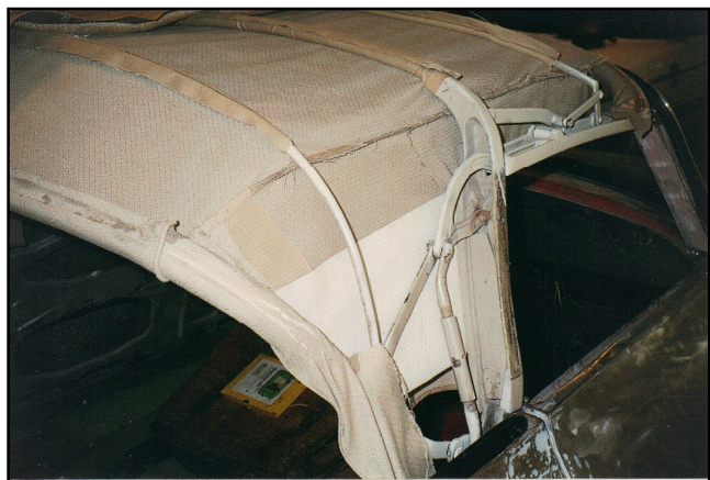
Aug. 2002 — The headliner attached to the refurbished frame
