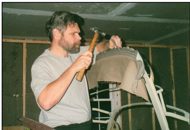
Nov. 2001— Attaching the guide rails to the header bow.
