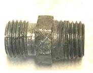
orange filter out to inspect and discovered that there was a crack in the small connecter where the oil line attached. In all these years I have never seen one crack but there it was and needed replacing. I went to the other engine, pulled the fitting off the silver canister, installed it and problem solved. Easy fix.
