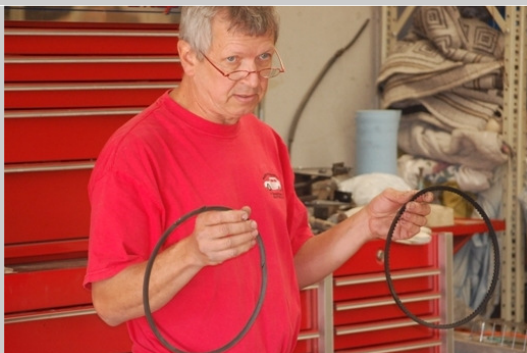
Rainer suggests regular fanbelt replacement, don't wait until it looks bad or breaks
