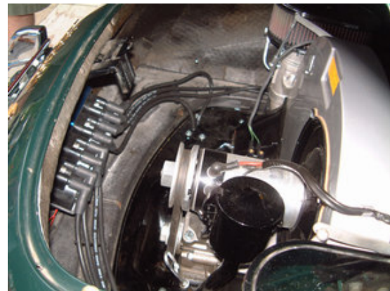
McManus' engine compartment – lots of wires, no distributor
