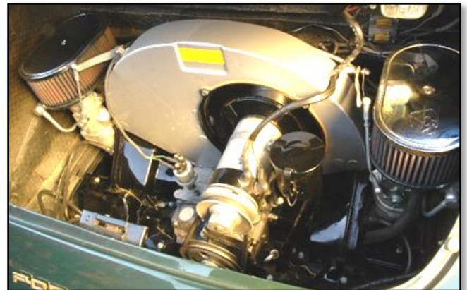
Engine installed in the 356 / note, no distributor or oil filter / full flow oil filter under left wheel well and electronic ignition
