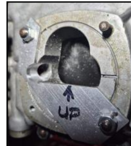
Figure 4 - Template provided to locate the ground notch.
