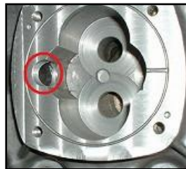
Figure 3—Location of the notch to be ground in the case.
