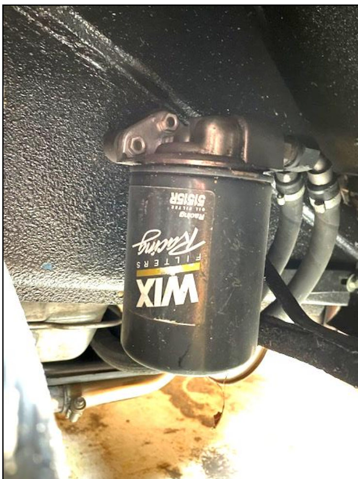
Figure 8—The Willhoit filter assemble mounted in the left rear wheel well of Mike's 356. The following are Mike's comments about the unit.
