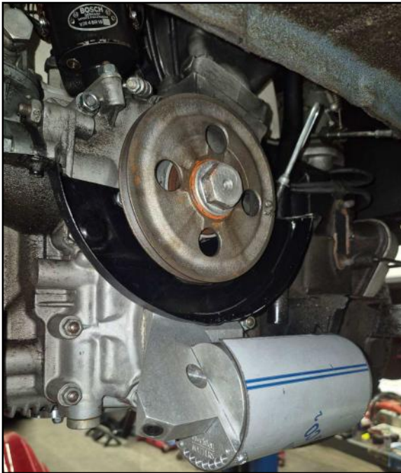
Figure 3—Location of the notch to be ground in the case.
