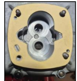
Figure 5 – The flow directing elbow assembled in the ground notch.
