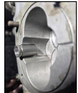
Figure 5 – The flow directing elbow assembled in the ground notch.
