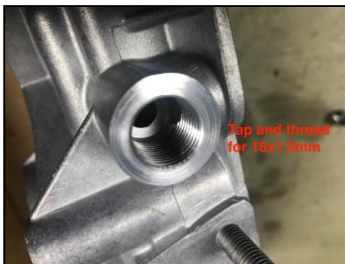
Above— Machining operations to install the unit
