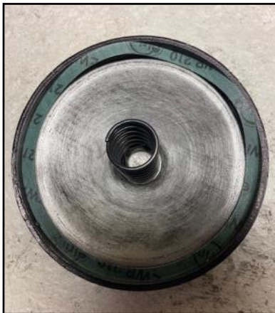
Above- Fram cover with gasket that came with oil filter.
