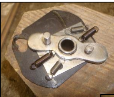
Above and right- Original 022 slip disc and the new Stoddard replacement springs (note original has ~22 turns, new has ~20 turns, both same end to end length)
