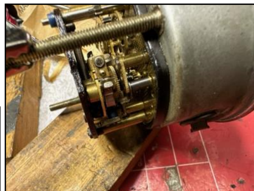
#4 Below—Bottom of mechanism shows the wide open point set on the 356B clock. When the points spark, the points open wide, thus winding the clock mechanism which ticks off until the points touch and spark open again. This is what enables our clocks to keep time.
