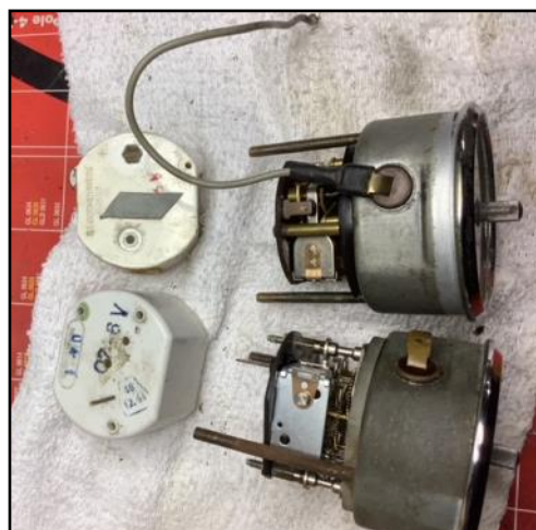
#5 right -Displays the half of point set removed from solenoid encasement. The thin copper piece with 90 degree bend was cracked through from wear and I had to solder it to conduct electrical current. You can see the solenoid exposed in picture #1. The copper piece is held in place by the two metal screws and the square cover.
