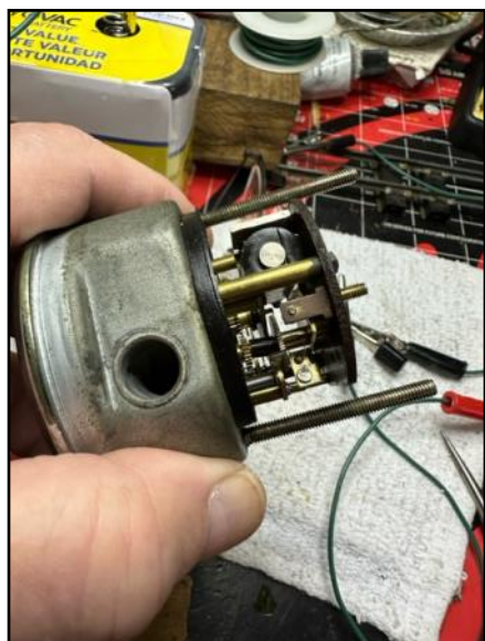
#1 left - Shows round, solenoid with metal actuator plunger in the center. Half the point set has been removed to gain access for solenoid replacement
