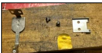
#5 right -Displays the half of point set removed from solenoid encasement. The thin copper piece with 90 degree bend was cracked through from wear and I had to solder it to conduct electrical current. You can see the solenoid exposed in picture #1. The copper piece is held in place by the two metal screws and the square cover.
