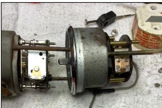
#4 Below—Bottom of mechanism shows the wide open point set on the 356B clock. When the points spark, the points open wide, thus winding the clock mechanism which ticks off until the points touch and spark open again. This is what enables our clocks to keep time.
