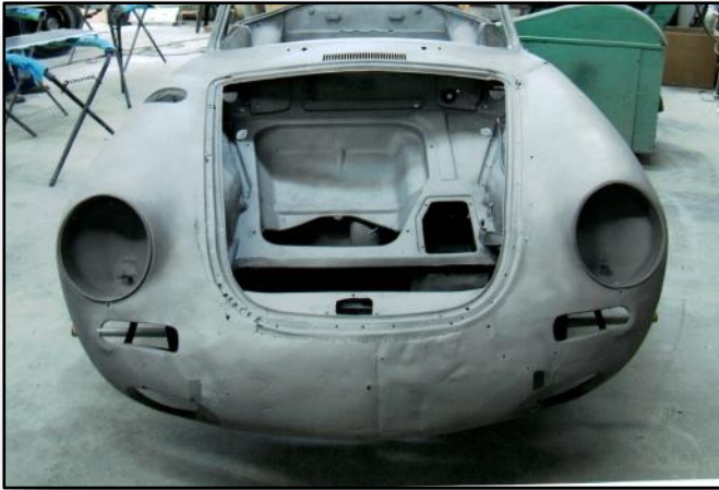
Above- Damaged nose and rotted rain gutter.
