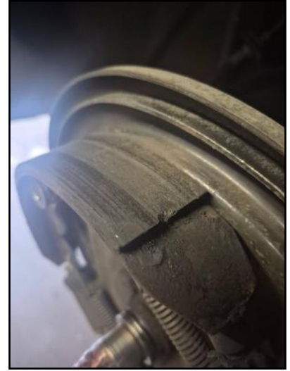
Above- Picture 4 Bad front lining
