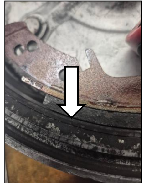
Right- Picture 7 Lining in contact with drum on the ends
