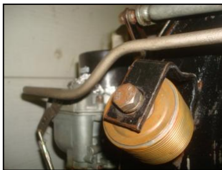
Above— Carl's engine showing the gas line passing over the bellows bracket.
