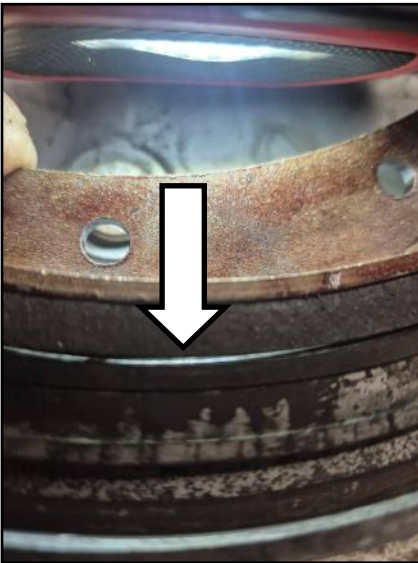
Left- Picture 8 Lining/drum gap in the center
