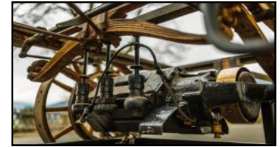
Above -The 1898 Egger-Lohner Chase Two (C2) in the Porsche Museum and view of the electric motor.
