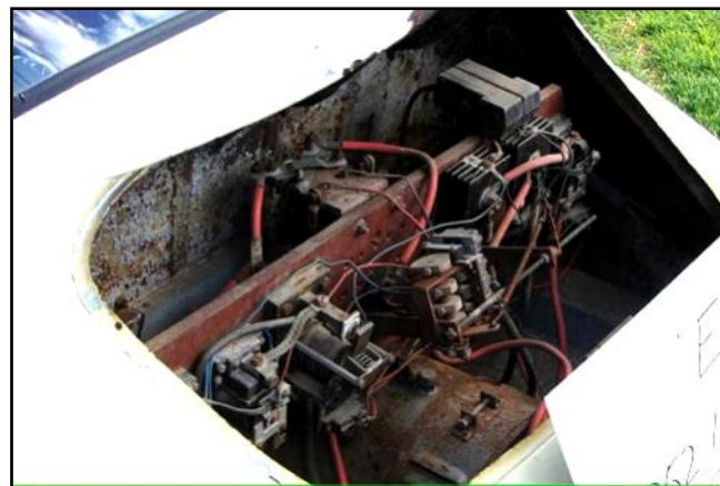
Above- you can see that the engine & fuel system were removed and a small DC motor & rear batteries installed. The top speed was 56 mph. Hal drove the car for 15 yrs in all types of weather in Pennsylvania until 1975.
